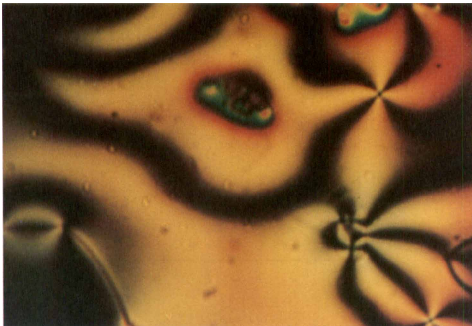
Figure 2. Optical micrograph showing the schlieren threaded texture of the nematic mesophase in FeESADCn ( n=6 ) at 451 K (heating cycle).
